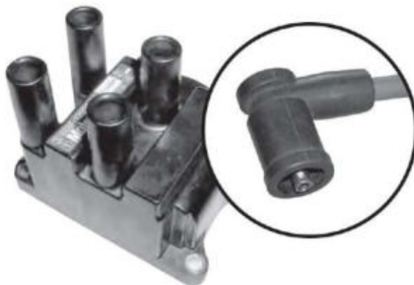
FORD 2nd GENERATION COIL PACK AND BOOT TYPE CONNECTOR
