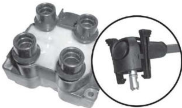
FORD 1st GENERATION COIL PACK AND CLIP/HOOK CONNECTOR
